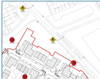
Figure 2-1 – Signage at pedestrian crossings
