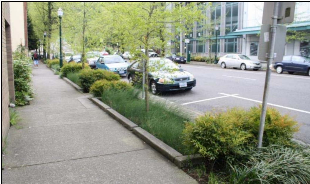
Figure 17: Reference image for verge as SuDS device (extract from SDDS)
