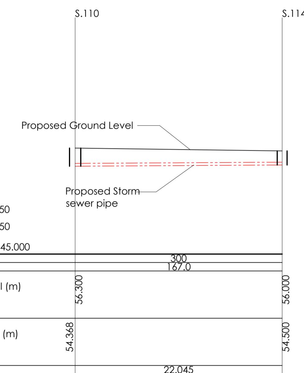
**Longitudinal Storm Sewer Section MH's S.110 - S.114**
