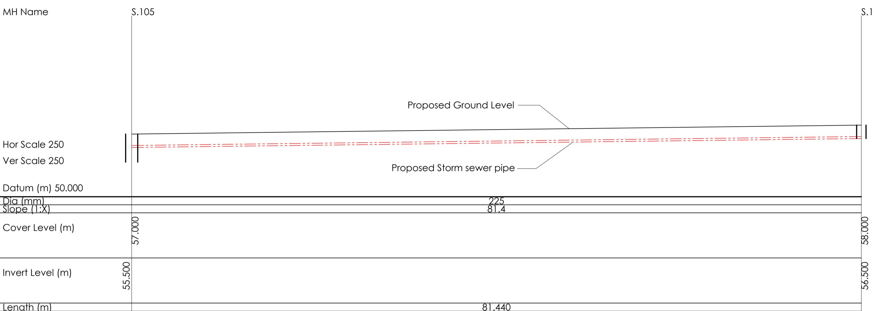
**Longitudinal Storm Sewer Section MH's S.105 - S.106**
