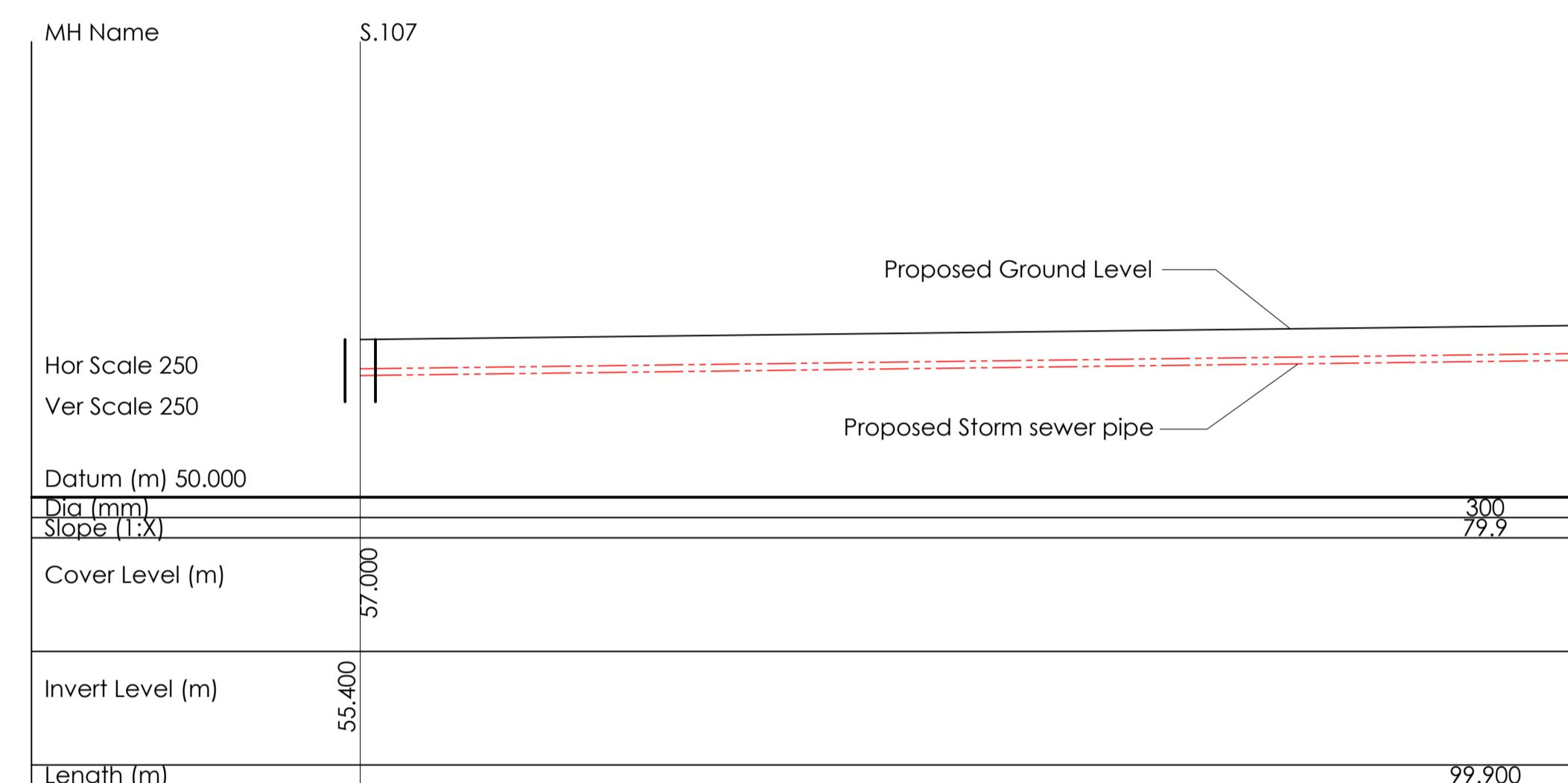
**Longitudinal Storm Sewer Section MH's S.107 - S.109**
