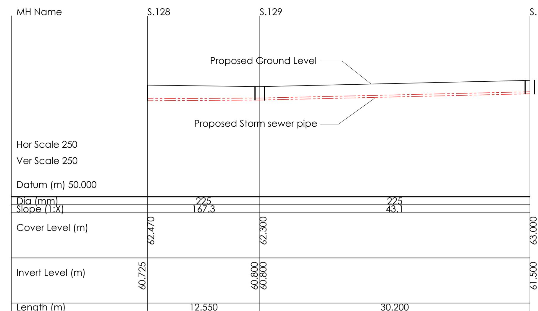
**Longitudinal Storm Sewer Section MH's S.128 - S.130**
