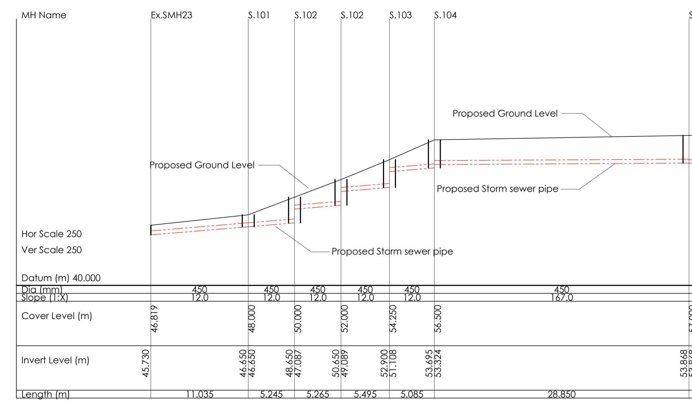
**Longitudinal Storm Sewer Section MH's ex.SMH23 - S.107**
