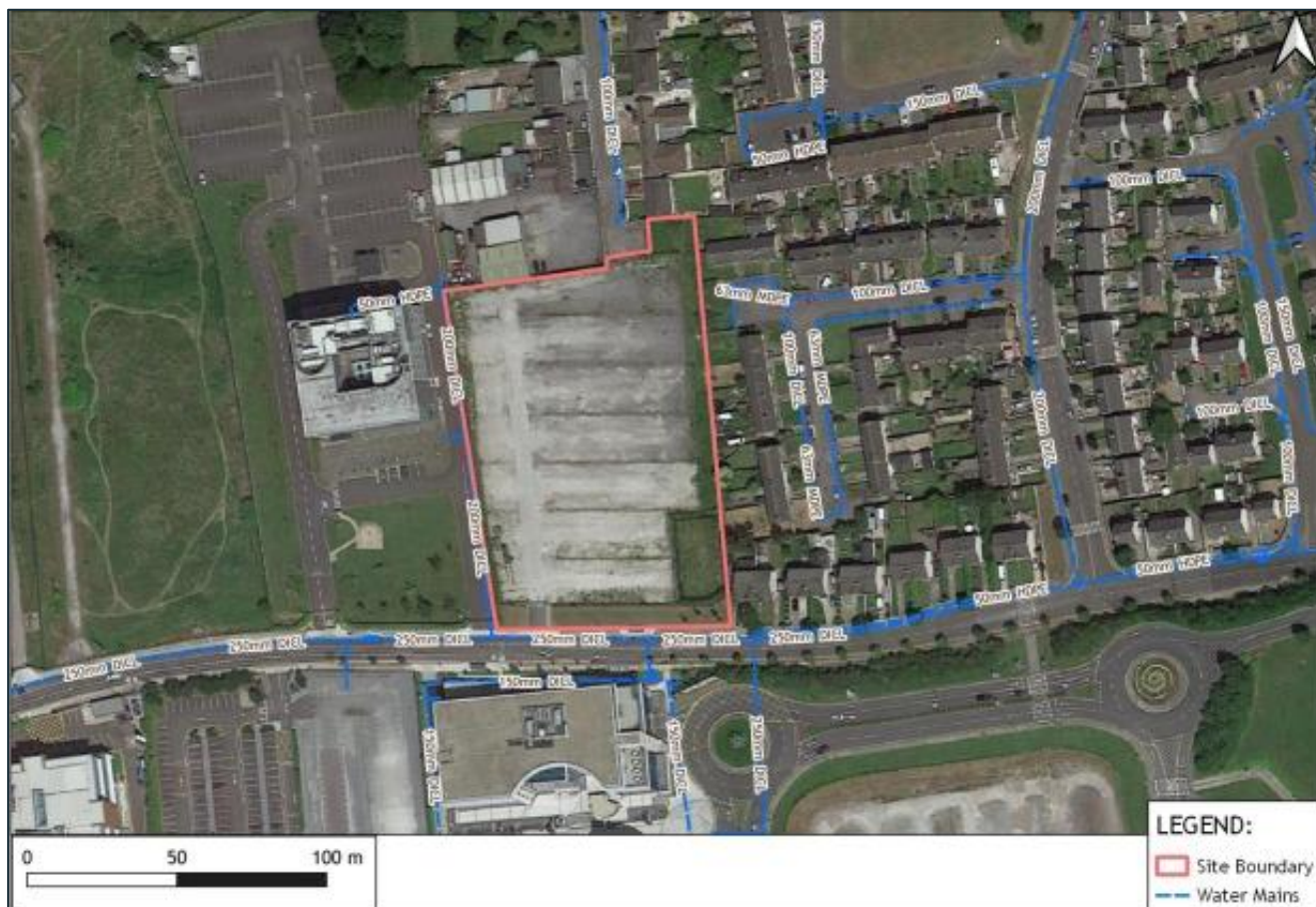
Figure 1.11 - Existing watermain connections surrounding the site (from Punch Consulting Engineers, 2024 (Extract from Uisce Éireann online records)).
