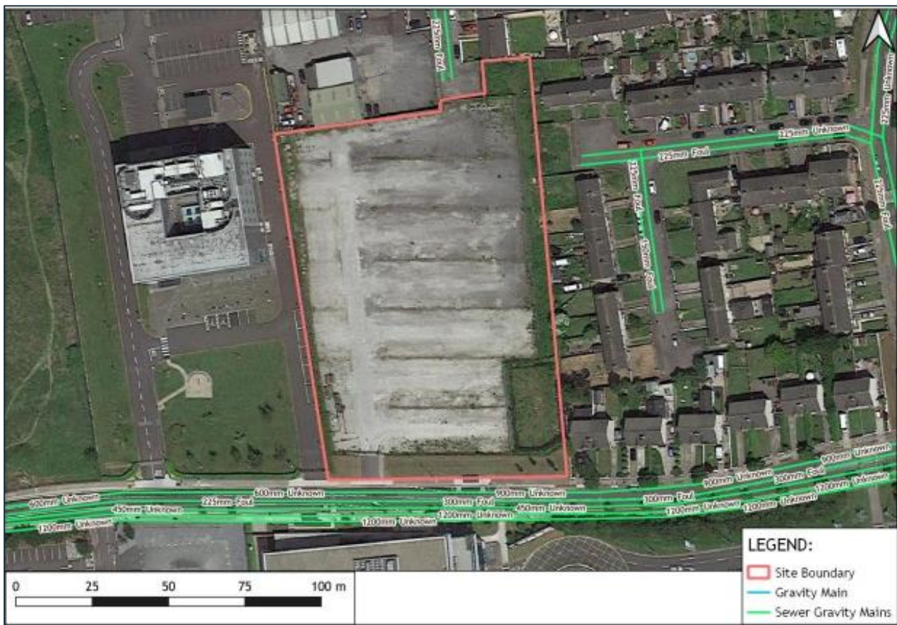
Figure 1.10 - Existing foul drainage surrounding the site (from Punch Consulting Engineers, 2024 (Extract from Uisce Éireann online records)).
