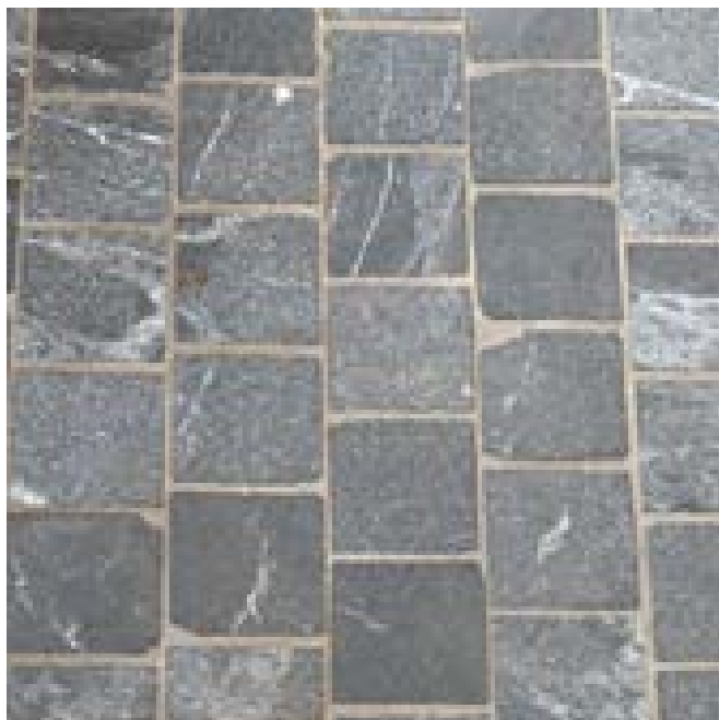
PAVING TYPE A: Granite Paving Setts Size: 150 x 150 x 150mm thickness 150 x 150 x 100mm at building threshold Colour: Dark Granite (G-B-006)
