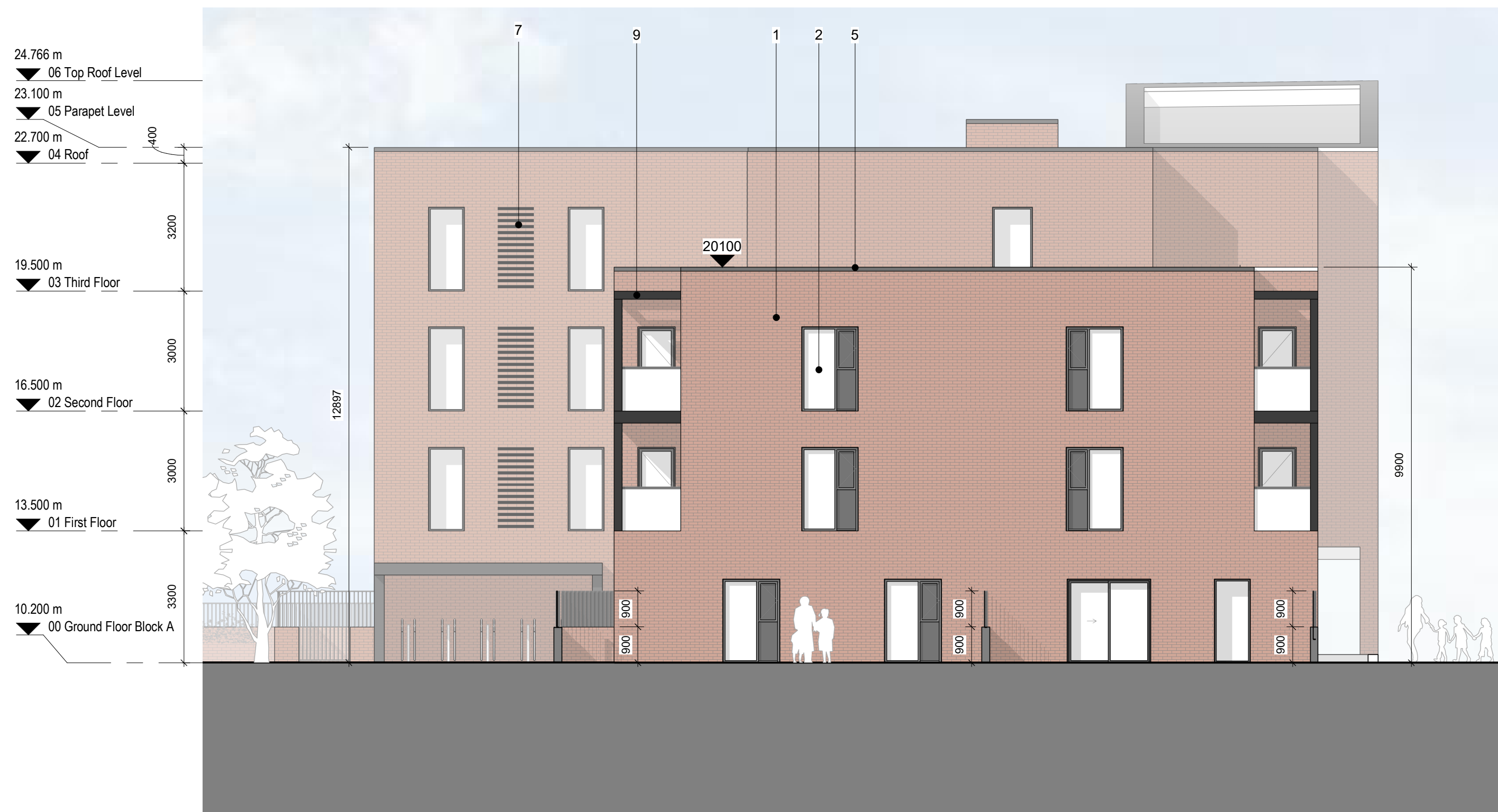
4 EAST ELEVATION BLOCK A 1:100
