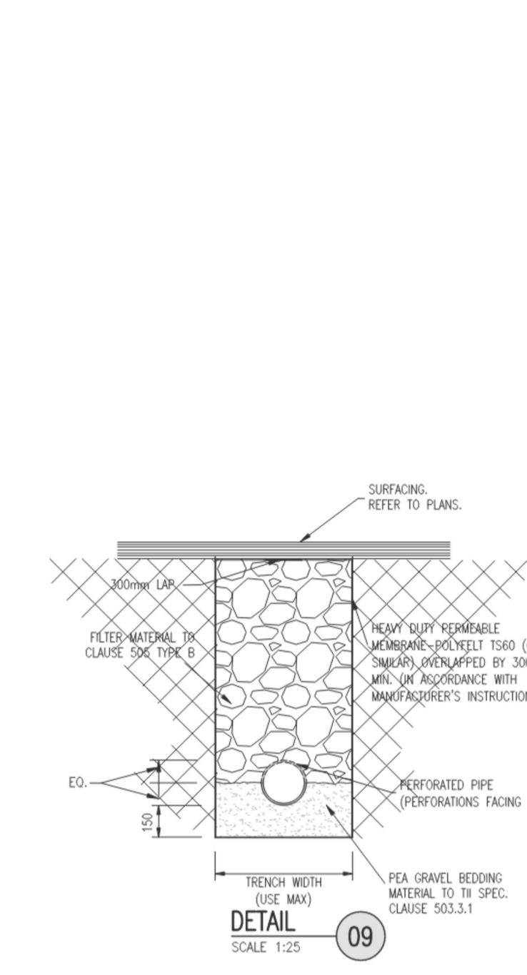
(TYPICAL) Filter Drain Detail
