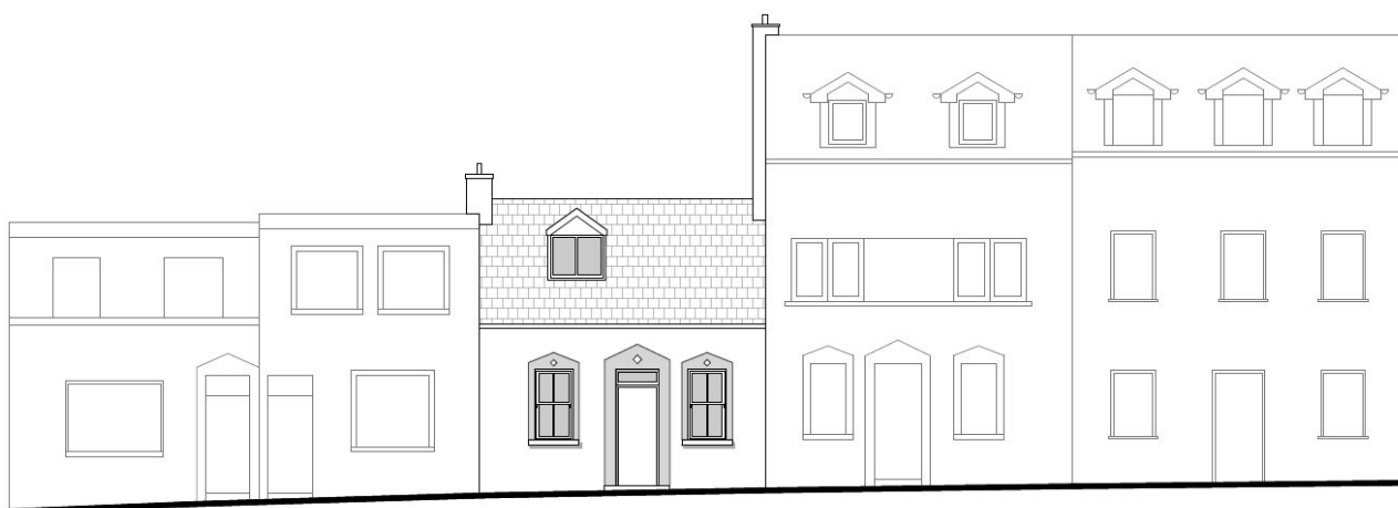
Fig. 13: Drawing of the existing front elevation of 38 Gould Street. The elevation is to be retained from eaves level down.
