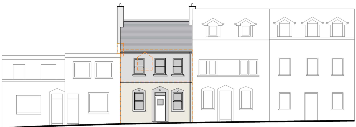
Fig.1.6: A drawing of the proposed elevation, illustrating the retention of the existing ground-floor façade.
