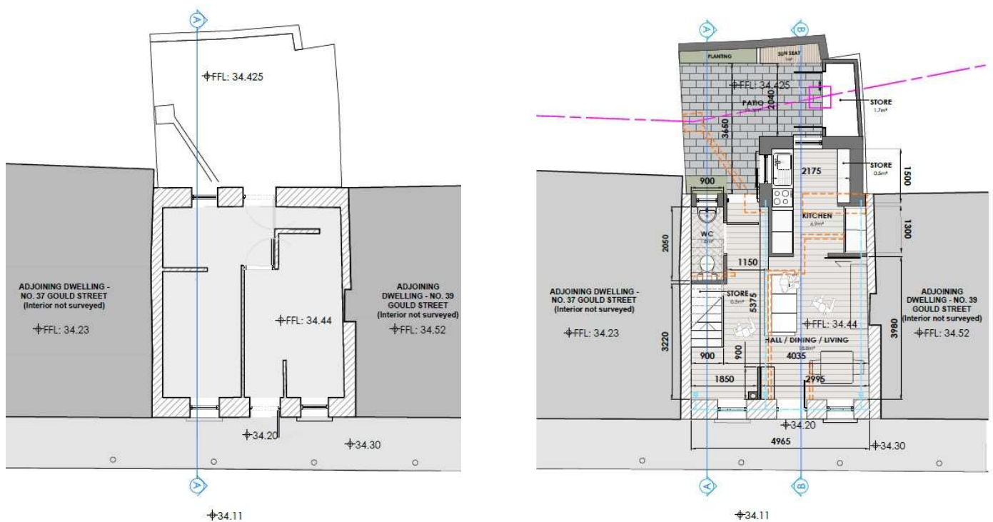
Fig. 15: The existing floorplan in comparison to the proposed floorplan – demonstrating the retention of the front façade and the proposed extension behind it.
