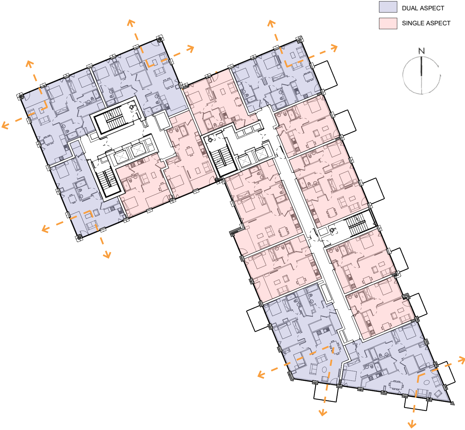
Image 3.32 General floor plan layout showing dual aspect units
