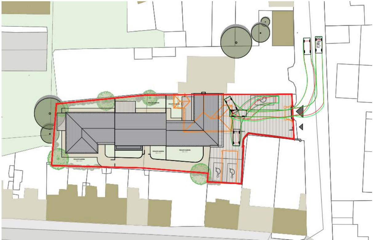
Fig. 21a: Turning analysis of the proposed parking space 1.
